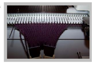
Now knit moving the carriage to the left. The needle in hold should not knit and the yarn will be going over the needle. You will now manually place the yarn under the needle. This is called wrapping the stitch. See photo on right.
