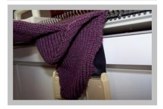
Ribbing - Now you are back up to the ribbing. You are finished hanging the side stitches. Knit 20 rows and latch back up for ribbing.
