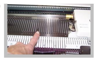
Note: As you are increasing your short rows out. You need to move your claw weight up about every other row to keep the stitches from dropping off the needles. As you knit the heel of the sock, a pocket will form. You need to keep the weight on these stitches.
