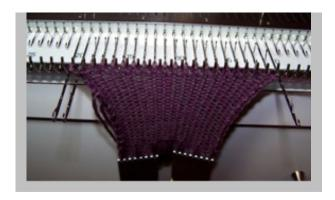
Knit, moving the carriage to the left. Wrap the yarn under the second to end left needle. See photo on right.
